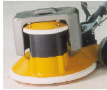
Machine with cast aluminium housing and saddle weight
