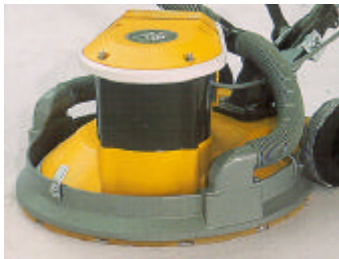
Grinding with dust control
